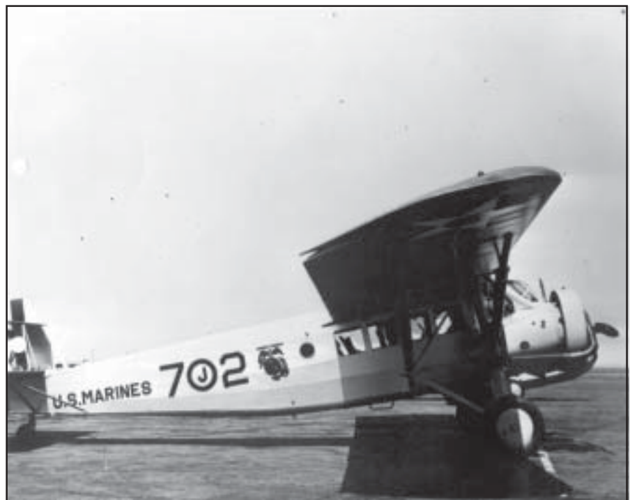
RC-1 Transport Ambulance, twin-engine, 2 crew, land, monoplane "Kingbird" by Curtiss-Wright. Defense Dept. Photo (Marine Corps) 517611
